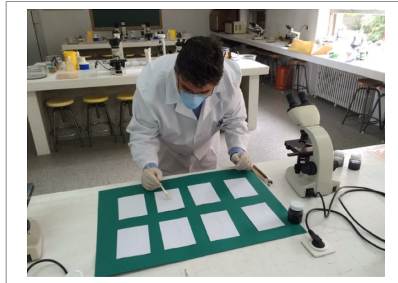
Figure 1. Tests on antibacterial paints doped with graphene at the Construction Science Institute Eduardo Torroja
