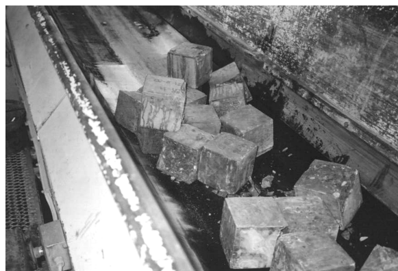
Figure 3. Test cubes before being crushed
